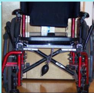
Wheelchair Seat Insert Frame without cushion. Adjustable Adaptor pan to mount seat to different wheelchair frames Hand Pump to allow stiffness of HT resistance to be adjusted.
